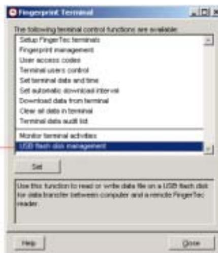
Double click **USB flash disk management** to start the USB Management in FingerTec® Biometric Settings.
